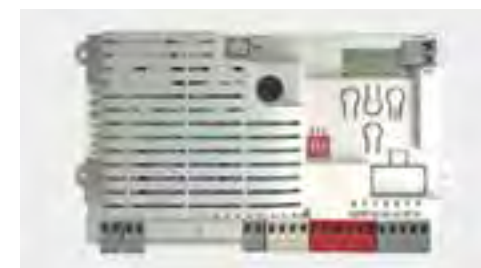
New control unit CTE20324 with integrated receiver programmable with KUBEPROW
