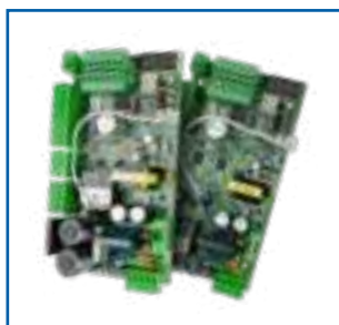
Next-generation EVO control board, compliant with EU Regulation 2023/826, ensuring stand-by consumption below 0.5 W
